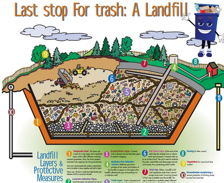
and regulations state that it cannot accept more trash, it must be closed cap is made from a synthetic plastic followed by a four fact knyer of dist. Once and shallow rooted plants are planted on top to prevent the erosion of the soil cap.
